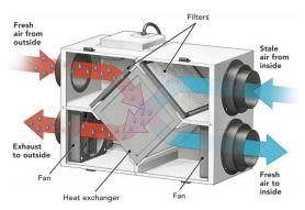
occupants' comfort is also increased as the air supply is warmed before entering the rooms. The MVHR unit which houses the heat exchanger and the fans is also equipped with filters which prevent outside dust entering the system and internal air particles depositing within the unit.
